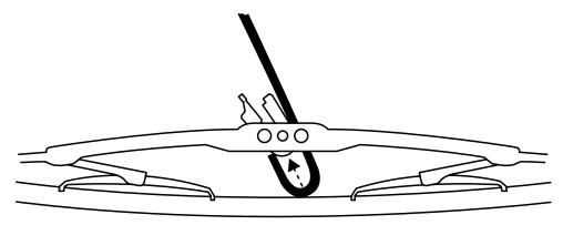
6. Determine your preferred windshield wiper park position with wiper blade parallel to vertical window edge. Loosen set screw in arm mounting head. To install wiper arm, place arm mounting head over pivot shaft with arm in desired park position and tighten set screw to 4.5 Nm (40 lb.in).
